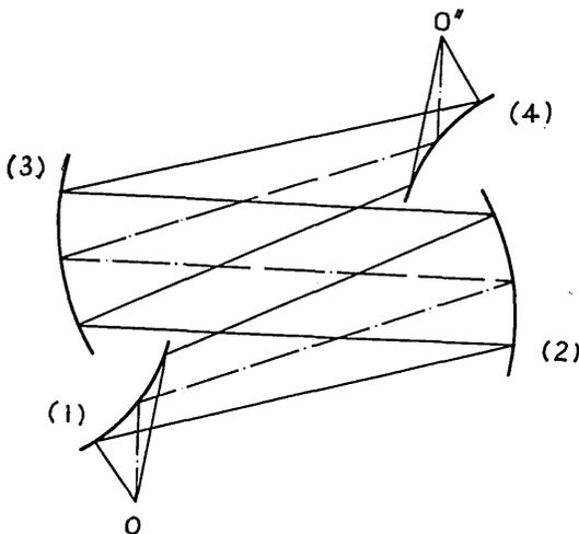
FIG. 3. Czerny-Turner arrangement with compensation for astigmatism.
